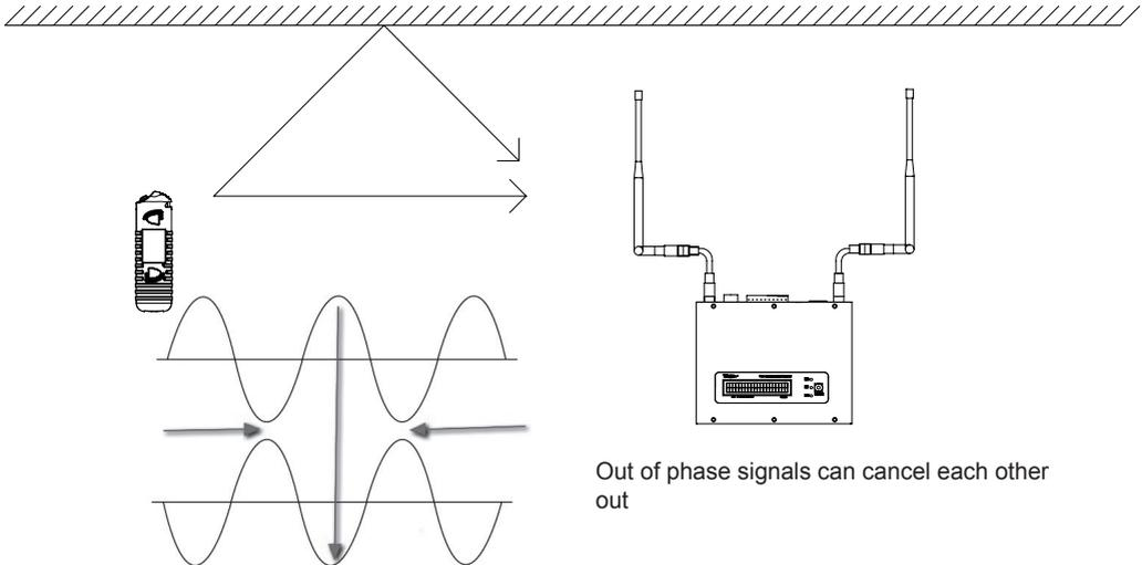
For optimum signal coverage when using either the Omni or Directional antenna they should be:
