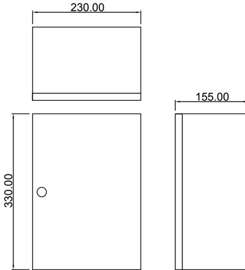
**T101 Single Receiver mounted in IP65 Box with microphone**
