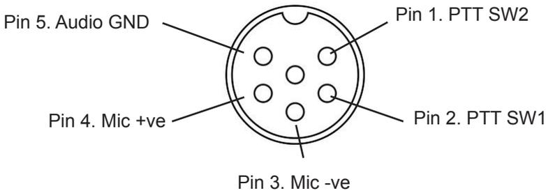
Wired PTT microphone via 5pin 240degree locking Din. Preh part no 71430-250/0802
